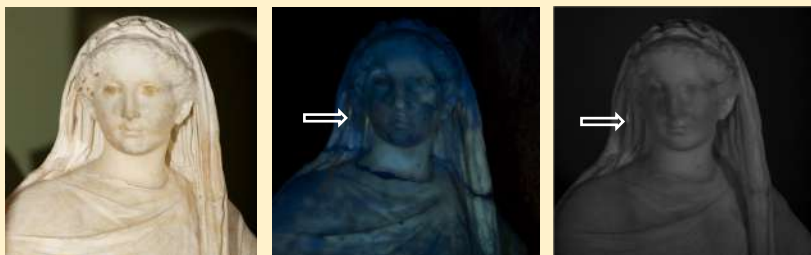
Visible, UVL and VIL images indicating the coexistence of a red lake and Egyptian blue
